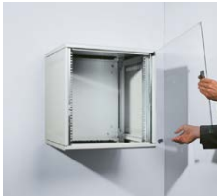
Mount the 482.6 mm (19") angles in the required position and slide the left and right hand side panels into place. Then, install the glass door by inserting the hinge pin into the top drill hole first, before allowing the bottom pin to slide into the lower hole. Secure the door at the top with the red securing ring.
